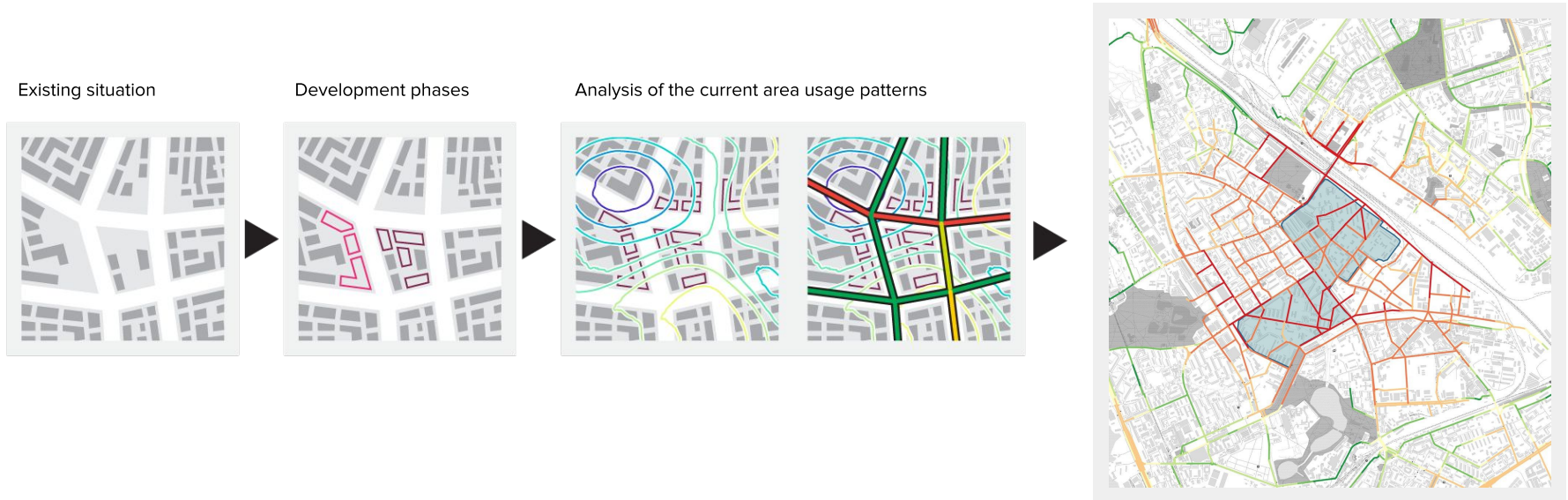
An example of connectivity modelling for a new development area on the periphery of Moscow
